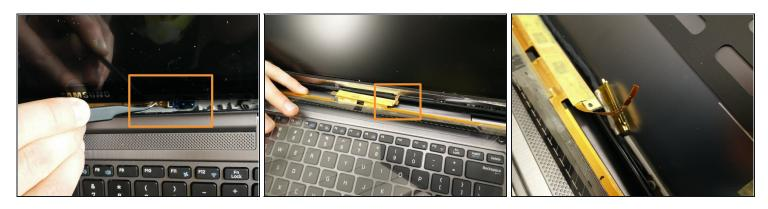
• There is a small, skinny wire leading from the bottom of the touchscreen to the joint of the laptop. Remove carefully with <u>tweezers</u>.
