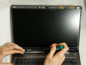
Unscrew the six 3.7 mm screws holding the screen in place.
