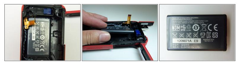
• After removing the battery housing, take the battery out.
