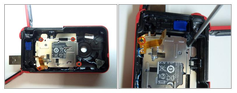
• Remove the four screws from the battery housing using a Phillips #00 screwdriver.
