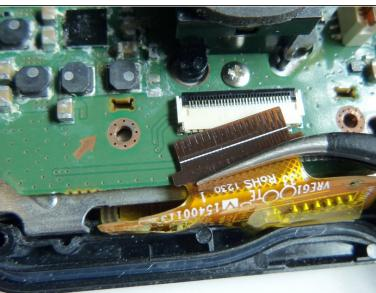
Use tweezers to grab the wire ribbon, then pull the wire out of connection.
