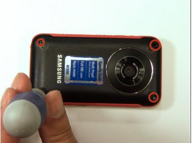
Remove four screws with a Hex 1.5 mm screwdriver.
