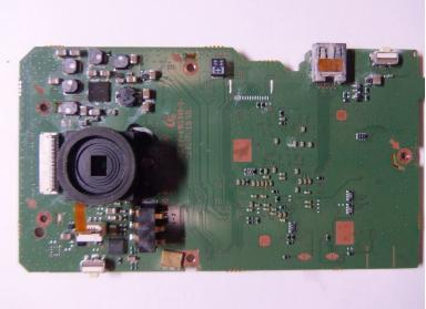
Use tweezers to disconnect the wire as shown. This will loosen the motherboard from the rear case.
