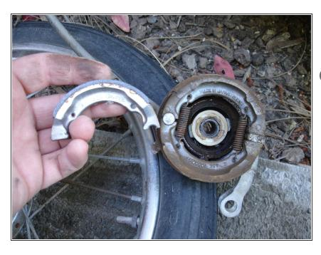
(i) A comparison of the old and new brake shoes. The old ones were worn to the bare metal at some points.
