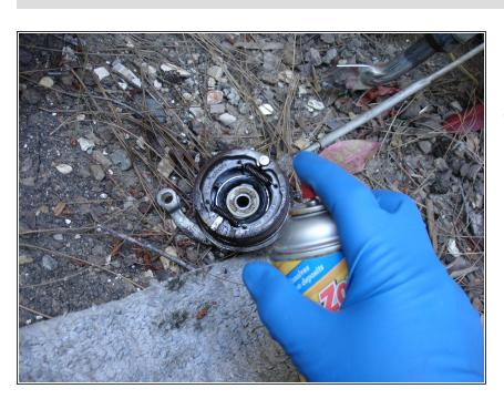
Spray all of the brake shoe hardware with the cleaning solvent before taking off the old shoes. This will clean the hardware and prevent any asbestos from flying into your lungs.
