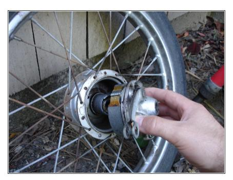
Place the brake drum assembly back into the wheel.
