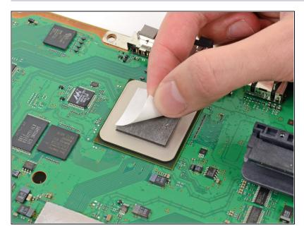
Peel the remaining white plastic cover off the other side of thermal pads.
