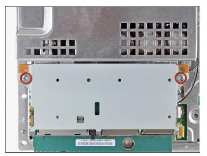
Remove the two 9 mm Phillips screws securing the memory card reader to the chassis.
