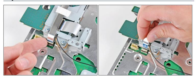
• Flip up the flap on the memory card reader ribbon cable socket and remove the ribbon cable.
