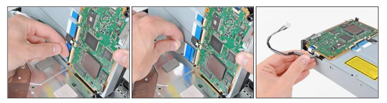
• Use your fingernail to flip up the retaining flap on the Blu-ray ribbon cable socket.
