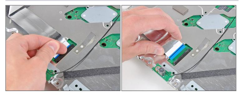
• Flip up the retaining flap on the Blu-ray ribbon cable socket.
