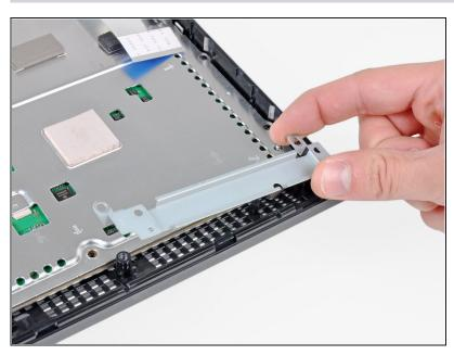
Remove the control board bracket.
