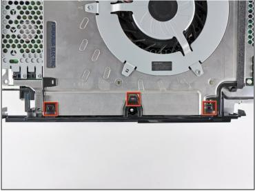
• While lightly pulling the rear cover away from the logic board assembly, use the flat end of a spudger to release the clips along the top and bottom edges of the rear cover.
