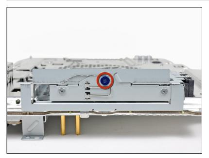
Remove the blue 8 mm Phillips screw securing the hard drive cage to the chassis.
