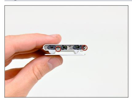
Remove the two Phillips screws on the controls side of the Shuffle.
