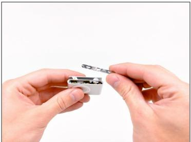
• Use the edge of an iPod opening tool to remove the steel plate from the controls side of the Shuffle.
