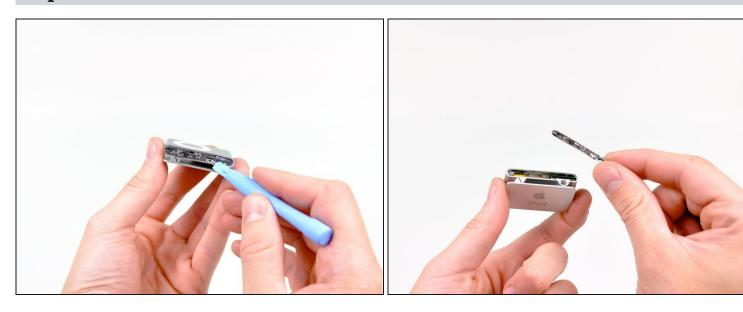
• Use the edge of an iPod opening tool to remove the steel cover from the headphone jack side of the Shuffle.
