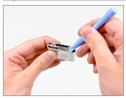
Use the edge of an iPod opening tool to slightly pry the steel plate on the headphone jack side of the Shuffle away from the lip cut into the outer case.
