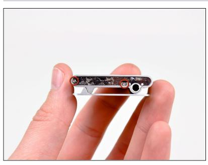
Remove the two Phillips screws from the headphone jack side of the Shuffle.
