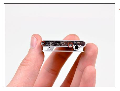
Remove the two Phillips screws from the headphone jack side of the Shuffle.
