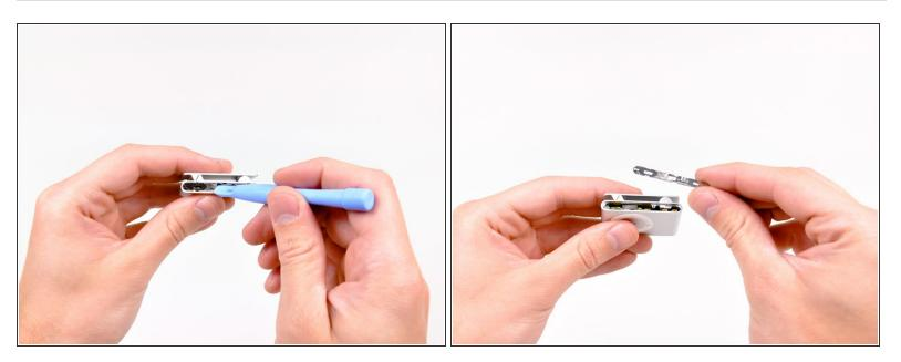
Use the edge of an iPod opening tool to remove the steel plate from the controls side of the Shuffle.
