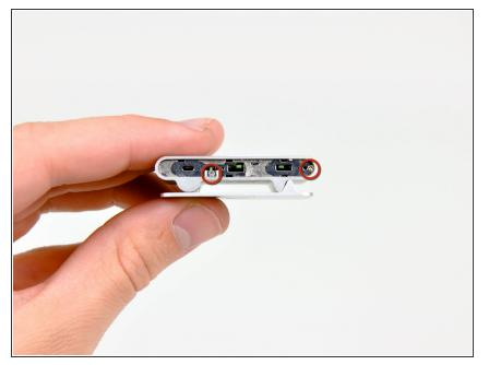
• Remove the two Phillips screws on the controls side of the Shuffle.
