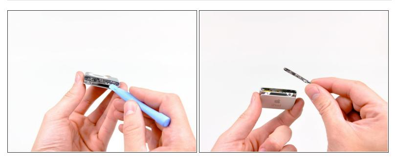
Use the edge of an iPod opening tool to remove the steel cover from the headphone jack side of the Shuffle.
