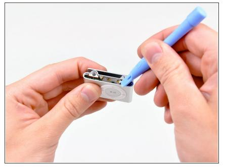
Use the edge of an iPod opening tool to slightly pry the steel plate on the headphone jack side of the Shuffle away from the lip cut into the outer case.
