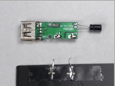
Solder the two contact points identified by the "S+" and "S-" to disconnect the USB assembly.
