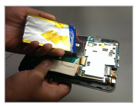
Fully remove the battery from the device.
