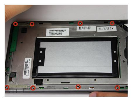
Remove the ten 4.0 mm screws from the device's perimeter using the T5 Torx screwdriver.
