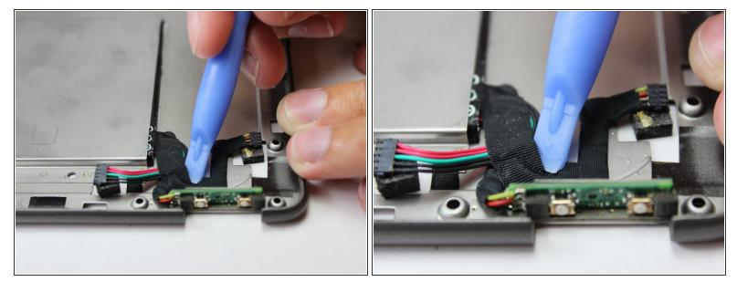
Remove the tape which holds the wiring to the battery using a plastic opening tool.
