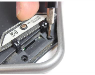
Remove the two 3.8 mm screws located in the back right corner of the device using the T5 Torx screwdriver.
