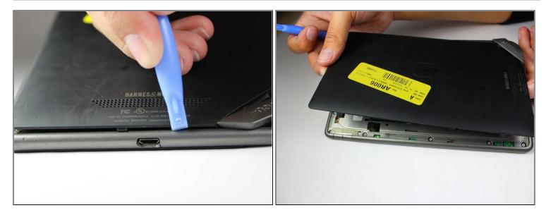
• Pry off the back cover with the plastic opening tool. Go around the device with the tool to ensure complete detachment.
