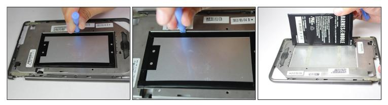
• On the back side of the middle panel, pry the battery using the plastic opening tools.
