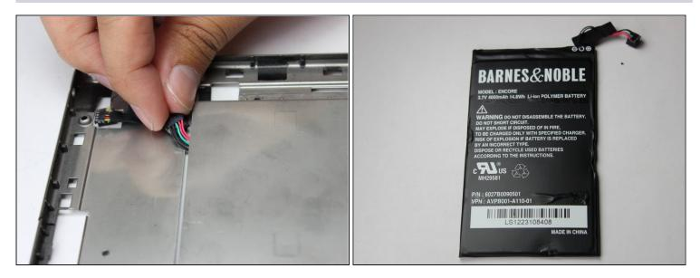
• Slide the connecting wire through the opening of where the battery was placed.
