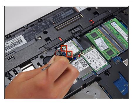
Lift up the two tabs connected to wires.
