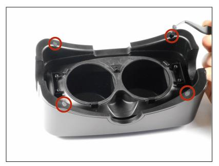
Using tweezers, carefully lift the four rubber plugs as shown. They are a bit snug and you may need to jiggle them free with the tweezers.
