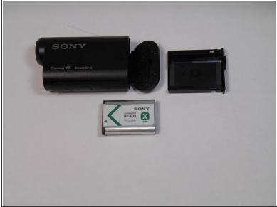
Using a pair of tweezers, firmly grip the protrusion where the PULL signifies and remove the tray and battery.
