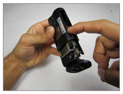
Separate the outer casing from the electronics by pushing on one of the ports toward the back end of the case. The electronics should slide right out.
