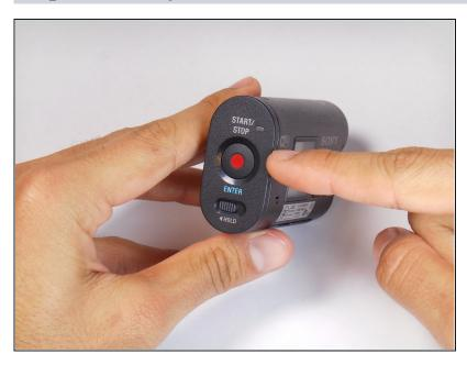
To access the battery, gently pry open the rear cover of the action cam.
