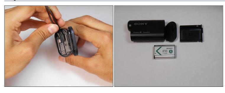
• Using a pair of <u>tweezers</u>, firmly grip the protrusion where the PULL signifies and remove the tray and battery.
