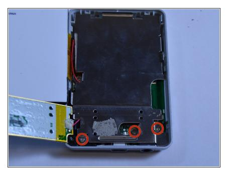
Use a Phillips Head screwdriver to unscrew the three 3/16 inch screws that were underneath the button input chip.
