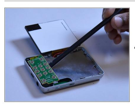
Using a spudger, pry off the button input chip from the mid-section of the device. To gain best leverage,
