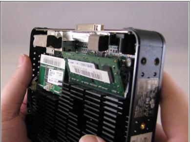
Using fingers, push the clips on either side of the RAM. The RAM will pop up at a 45 degree angle when both clips are disengaged.
