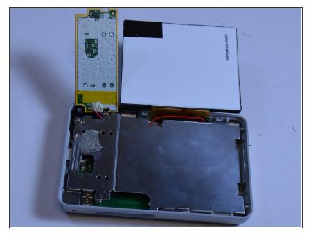
Lift open the LCD screen and button input chip to access the entire midsection plate.
