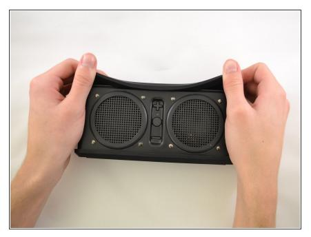
• Starting with the corners, gently pull the rubber cover off of the device.
