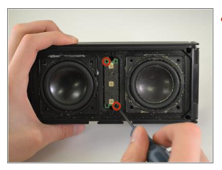
Using a Phillips #00 Precision Screwdriver, unscrew two 6 mm screws from the button motherboard.
