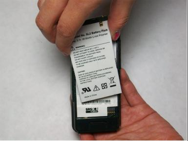
Pinch the battery from both sides and lift the battery to remove it.
