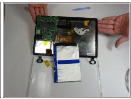
Carefully remove battery without putting any strain on connected wires. The battery is held to the tablet with adhesive, so be careful not to jerk the battery when it becomes loose.
