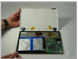
Take plastic opening tools, and find a spot on the back of tablet to lift the back plate. Once back is lifted enough, remove the back of the tablet carefully with fingers
