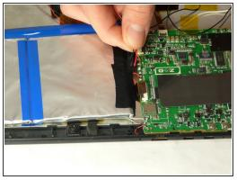
Use a soldering iron to carefully remove wires from motherboard. Then remove battery.
