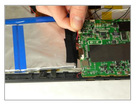
Locate battery, and examine wires connected to battery.
