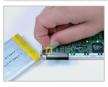
Carefully disconnect the white battery connector from the logic board. Be sure to pull only on the
