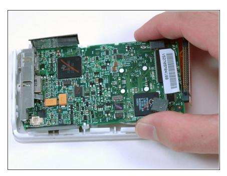
Slide the logic board away from the port end of the casing and lift it out of the iPod.
