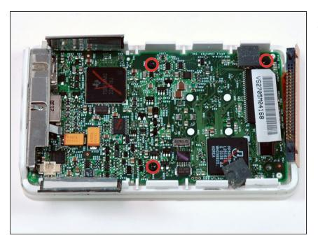
Remove the 3 remaining T6 Torx screws from the logic board.
