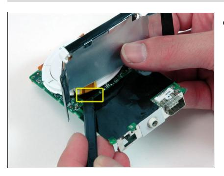
Use a spudger to carefully disconnect the display ribbon cable from beneath the scroll wheel.
