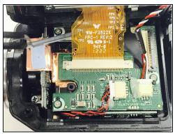
• Using the <u>tweezers</u>, carefully push up the left and right sides of the cable ribbon clip. Use the tweezers to life up and remove the clip.
