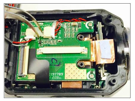
Turn the camera 180 degrees, and gently remove the glue from the connector as shown in the photo.
