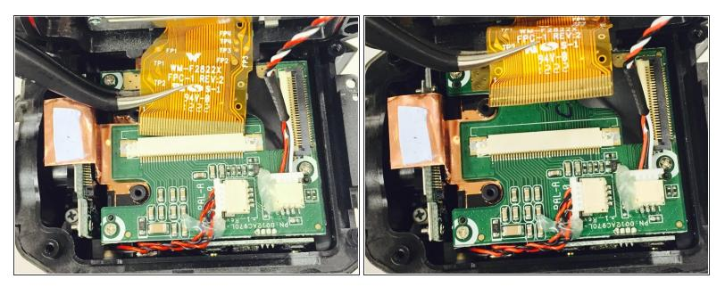
• Using the tweezers, carefully remove the ribbon cable by gently grasping it and pulling up.
