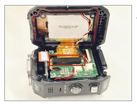
• Carefully lift open the camera from the side of the device with the record and play buttons. Then remove the black cover tape by gently peeling it off. Make sure to save this tape as you may need it when you re-assemble the device.
