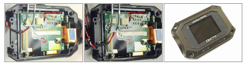
Now take out the connector by pulling the white clip out of the casing (as shown in the photos). This will will disconnect the screen from the main cable, allowing you to attach your new LCD cover.
