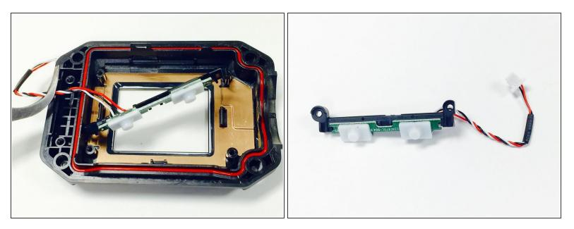
• The zoom (+/-) buttons are attached to the red, black, and white threaded wire. Use the tweezers to gently pull on this wire and remove the zoom (+/-) buttons.
