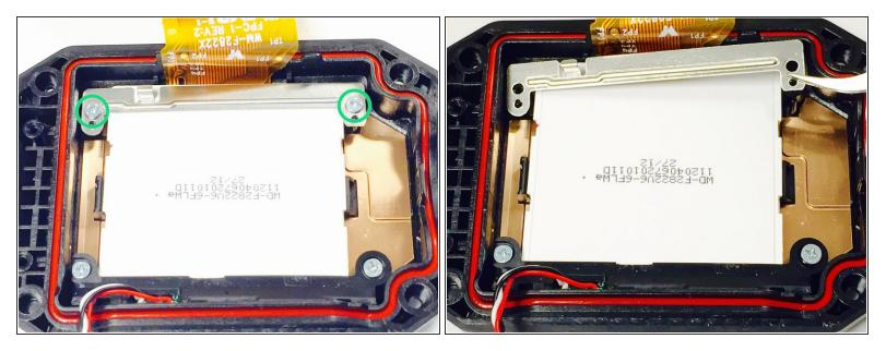
• Remove the top two Phillips screws (4mm headsize x 3mm length). Now use the tweezers to gently grab and remove the silver metal plate that the screws were holding in place.
