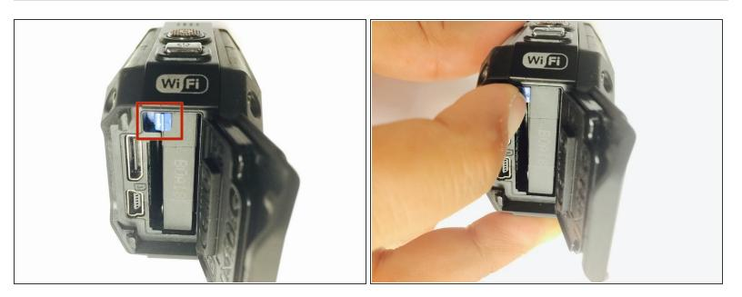
Push the cover up to open the battery compartment, and then push the blue battery release switch.
