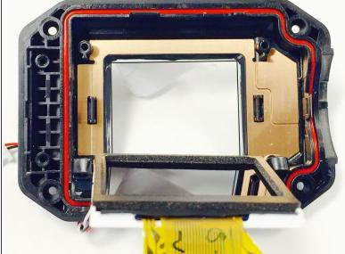
Using the tweezers, carefully lift up and remove the LCD screen.
