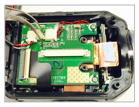
Turn the camera 180 degrees, and gently remove the glue from the connector as shown in the photo.
