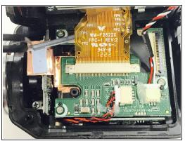
Using the tweezers, carefully push up the left and right sides of the cable ribbon clip. Use the tweezers to life up and remove the clip.
