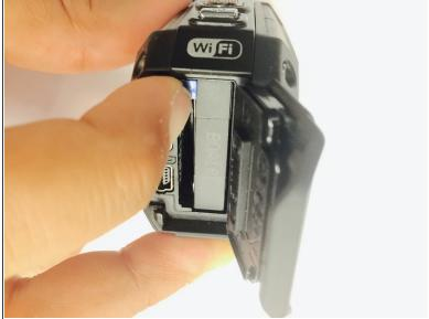
Push the cover up to open the battery compartment, and then push the blue battery release switch.
