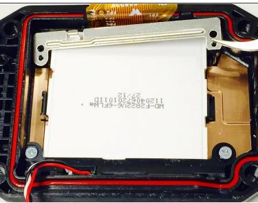
Remove the top two Phillips screws (4mm headsize x 3mm length). Now use the tweezers to gently grab and remove the silver metal plate that the screws were holding in place.
