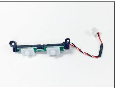
• The zoom (+/-) buttons are attached to the red, black, and white threaded wire. Use the tweezers to gently pull on this wire and remove the zoom (+/-) buttons.
