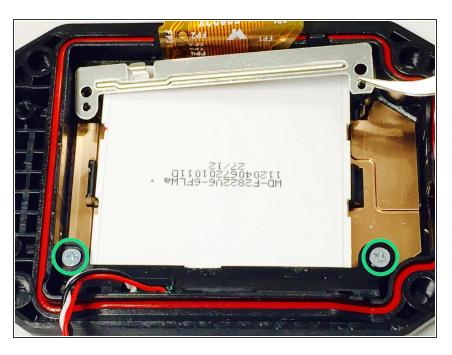
Remove the bottom two Phillips screws (4mm headsize x 3mm length).
