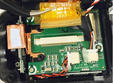
• Using the tweezers, carefully remove the ribbon cable by gently grasping it and pulling up.
