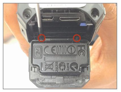
After removing the battery, take out the two Phillips screws (4mm headsize x 3mm length) screws. You can now remove the battery cover.
