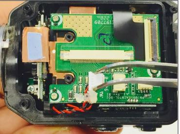
• Carefully peel off the glue holding the red and black braided wire down to the circuit board. Then remove the connector by gently pulling it out of its casing. You will want to save this glue as it may come in handy when re-assembling your device.
