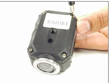
• Using a 1x1xH1.5 torx screwdriver, remove the 8 screws (5mm headsize / 4mm length) from the corners of both the front and back of the camera (4 screws on each side).
