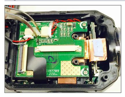
Turn the camera 180 degrees, and gently remove the glue from the connector as shown in the photo. Make sure you save the glue as you may need it when re-assembling your device.
