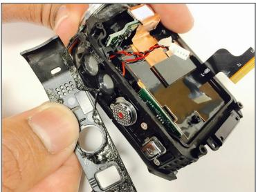
• Use the plastic opening tool to gently remove the top cover from the camera. It is glued on, so you may need to work at it to get it to come off.
