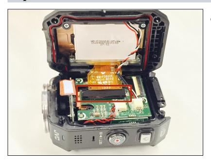
• Carefully lift open the camera from the side of the device with the record and play buttons. Then remove the black cover tape by gently peeling it off. Make sure to save this tape as you may need it when you re-assemble the device.
