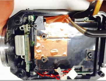
• Carefully remove both the top and bottom copper strips by gently pulling them off with the <u>tweezers</u>.
