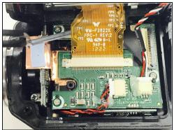
• Using the <u>tweezers</u>, carefully push up the left and right sides of the cable ribbon clip. Use the tweezers to life up and remove the clip.
