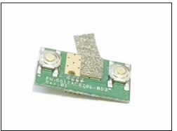
The power and record buttons are glued to the battery housing, so use the plastic opening tool to gently pry off and remove the buttons.
