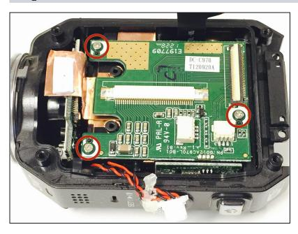
Remove the the three Phillips screws (3mm headsize x 2mm length) from the circuit board. After you remove the screws, you can then remove the green circuit board by lifting it up out of the device case. You may want to use the plastic opening tool to get start lifting the circuit board.
