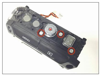
Once the cover has been removed, you will want to remove the three Phillips screws (2mm headsize x 2mm length) that are underneath.
