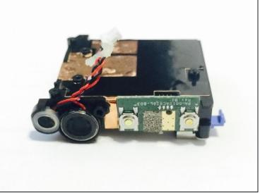
• Now you should be able to gently remove the battery housing out of the device. If you are having difficulty getting the battery housing to come out, you may want to use the plastic opening tool to help get it started.
