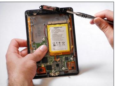
• Remove the magnetic component with the magnetic head of the aluminum driver.
