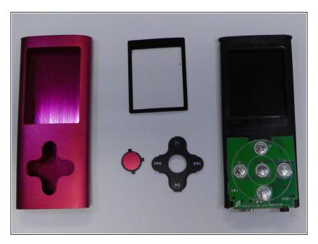
Freed from the internal space of the device, the LCD screen as well as the buttons will simply fall out of the face of the device. They can now easily be replaced.
