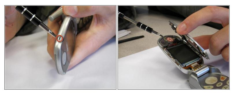
• Pry off the screen front cover with a small flathead screwdriver.
