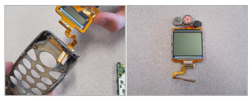
• Remove the LCD Screen from the phone case and replace with a new LCD screen.
