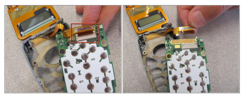
• Locate and detach the ribbon cable from circuit board.
