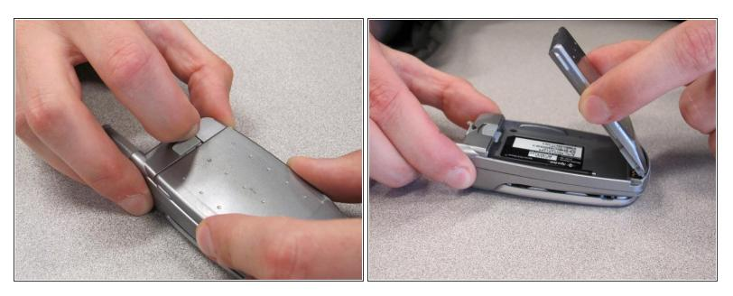
• While sliding the gray tab up, lift battery up and away from the cell phone.
