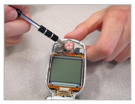
• Pry off the speaker which is glued on to the front cover using a small flathead screwdriver.
