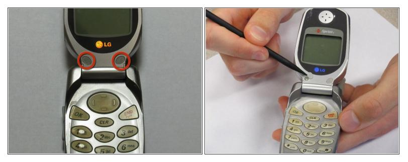
• Use a Spudger to remove the two front plastic covers to reveal screws.
