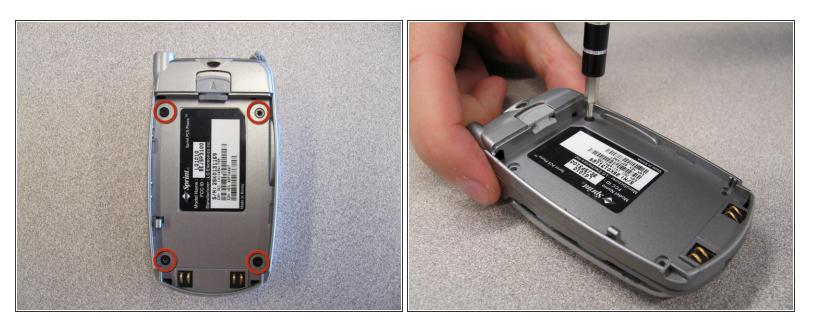
Unscrew the four screws on the back case using a T6 Torx Screwdriver.
