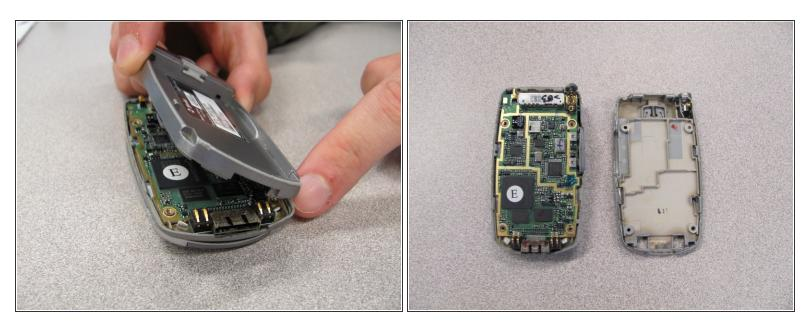
• Pull the back cover straight off the phone using your thumb and forefinger.
