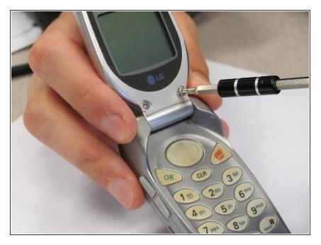
Remove two screws using a Torx T6 screwdriver.
