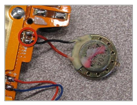
Obtain replacement speaker and solder the new black and red wires back to the base of the screen.
