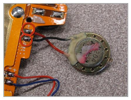
• Unsolder the black and red wires of the speaker from where they are attached to the base of the screen.
