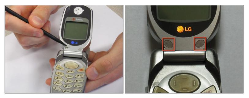
• Remove the two plastic screw covers below the inside phone screen.
