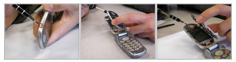
• Pry off the screen front cover with a 3mm flathead screwdriver.
