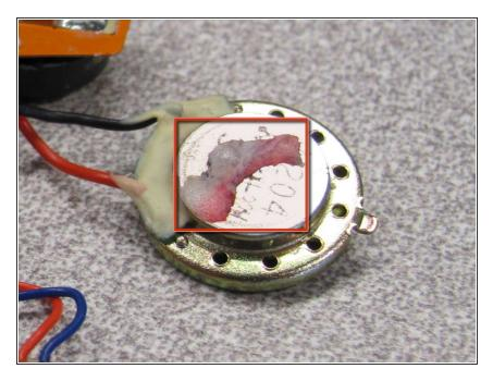
Apply glue to the back of the speaker and place it back in its original position.
