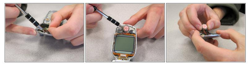
• Pry off the speaker, which is glued onto the front cover, using a small flathead screwdriver.
