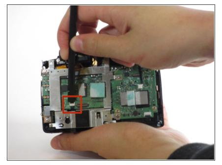
• Use a spudger to flip up the cable lock in order to release the ribbon.
