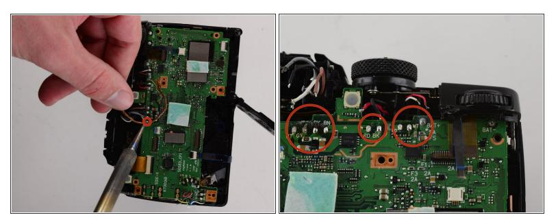
Desolder the labeled soldering points.
