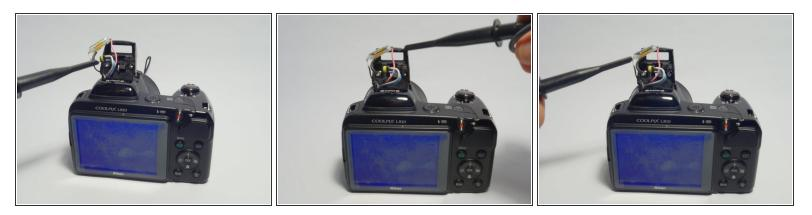
• Unsolder the wires that connect the flash component.
