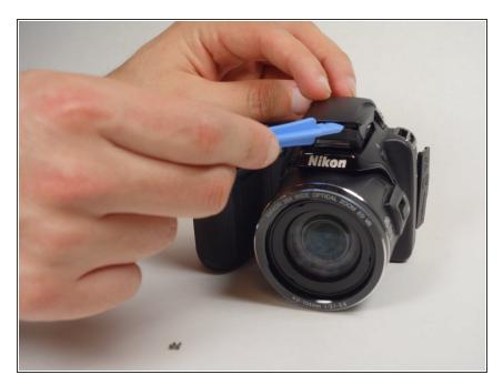
• Use blue plastic opening tool to pry open the casing for the flash.
