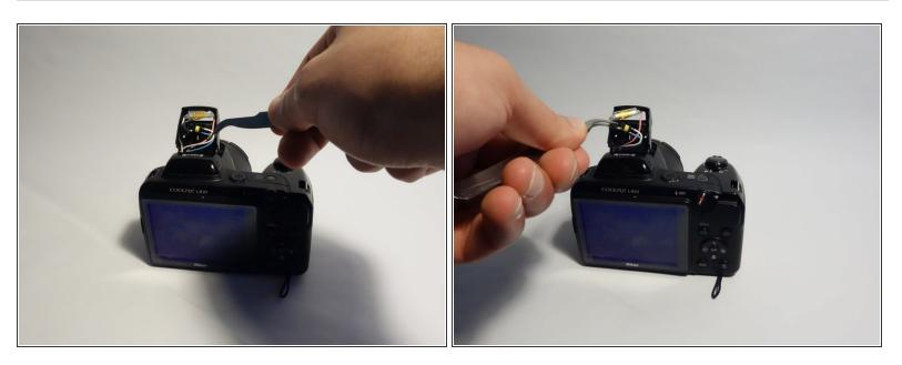
• Pull the wires connecting the flash out of the camera.
