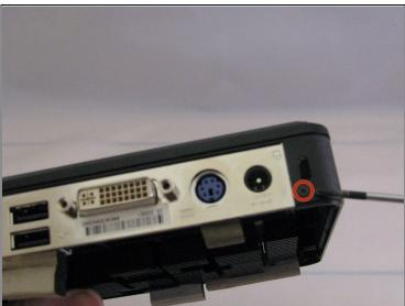
• Remove the two 4mm Phillips #00 screws that are along the back of the case.
