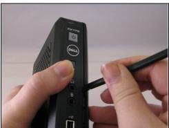
• Run the flat side of the spudger along the entire line of the case starting from the back where the power plug and a small screw are located.
