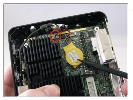
To remove the battery, pull up on the connector that is plugged into the motherboard.
