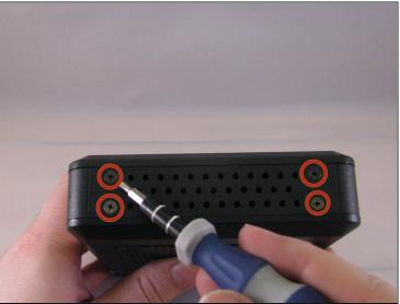
• Unscrew and remove the eight 4mm Phillips #0 screws (four on top, four on bottom) from the top and bottom of the device.
