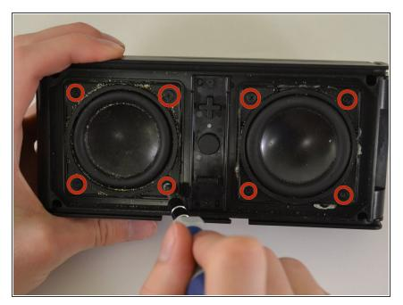
Using a #000 Philips Screwdriver, unscrew the four 8 mm Philips screws from each corner of both speakers (eight 8 mm Philips screws total).
