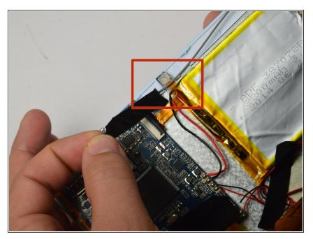
• Remove the tape that holds the camera in place.
