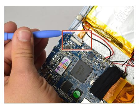
• Using the small plastic opening tool, gently push the gray connector back to unlock the flex cable.
