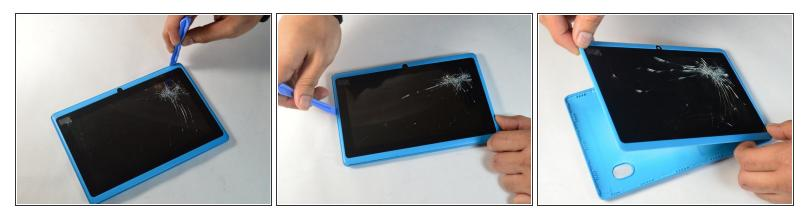
Place your Plastic Opening Tool between the screen and the case. Slowly move it around the casing while prying in a downward motion to undo the hinges holding the two together and separate the two parts.
