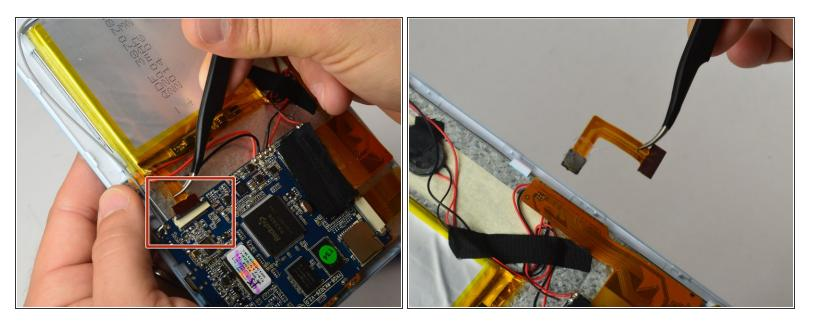
• Using a pair of tweezers, gently grasp the flex cable and pull it out while using your other hand to keep the camera in place. Once removed, your camera is now free and ready for replacement!
