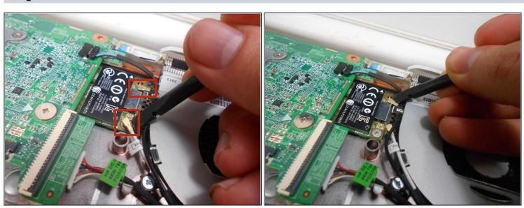
• Using a spudger, remove the white and black cables from the card.
