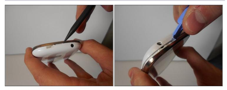
• Locate the small indent in the top of the device and use your nails or the plastic opening tool to separate the cover from the mid-frame.
