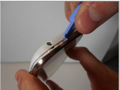
Locate the small indent in the top of the device and use your nails or a spudger to separate the backplate from the mid-frame.
