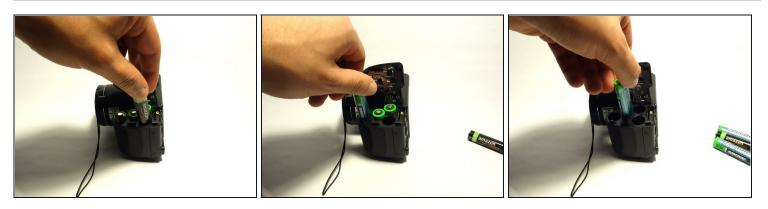
Remove four AA batteries one by one from the camera, making note of the proper alignment.
