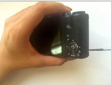
• Use the Phillips #00 screwdriver to remove the two screws located on the right side of the camera.
