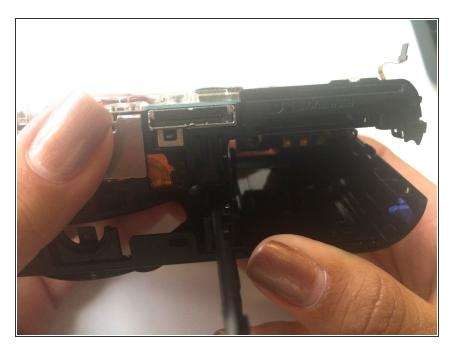
Pull off the front outer shell by pushing from the left side.
