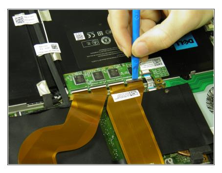
Use the opening tool's angled edge to lift the clasps securing the screen and motherboard cables.
