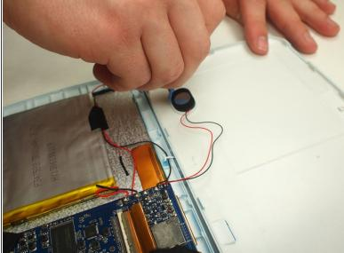
• Use the slim plastic opening tool to remove the speaker from its position on the case.
