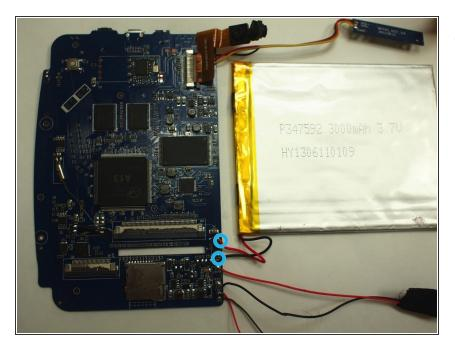
• Use the Soldering Iron to disconnect the each cable.
