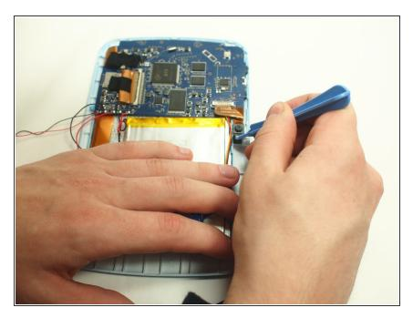
• Use the slim plastic opening tool to pry the camera from its initial position.
