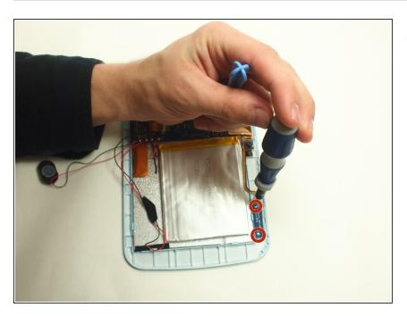
Remove the two screws that hold the volume button assembly in place.
