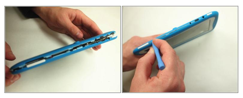
Slide the wide plastic opening tool across the seem, separating it if you can't pry the device open using just the spudger.
