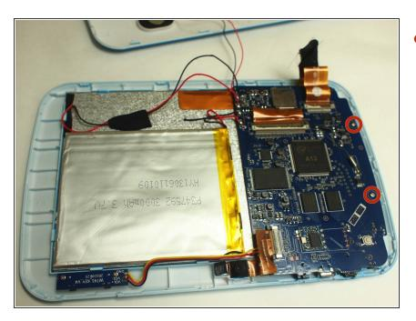
Remove screws located on the opposite side of the battery.
