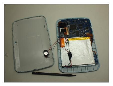
Locate the red and black wires that connect the speaker to the motherboard.
