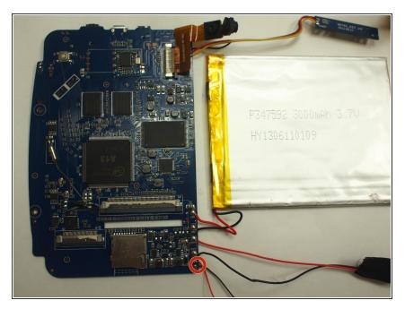
Un-solder the red and black speaker wires that are connected to the motherboard
