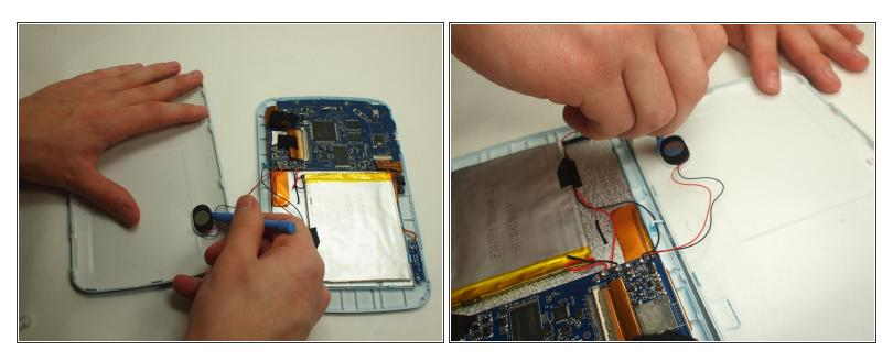
• Use the slim plastic opening tool to remove the speaker from its position on the case.
