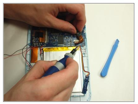
• Un-solder the yellow, red, and black wires that connect the volume module to the motherboard.
