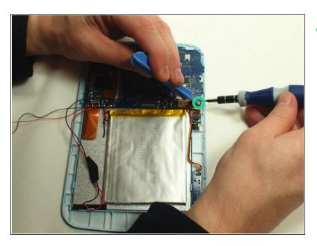
• After removing the camera, remove the hidden screw.
