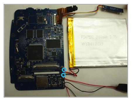
• Use the Soldering Iron to disconnect the each cable.
