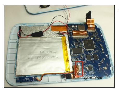
Use the precision tweezers to gently disconnect the camera ribbon that is connected to the motherboard.
