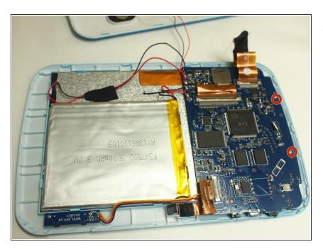
Use the screw driver to remove the highlighted screws.
