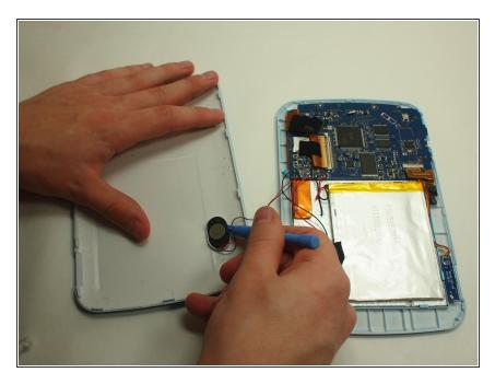
Use the plastic opening tool to remove the speaker from the casing.
