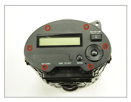
Using a Phillips head screwdriver, remove the six 4mm screws from the face of the camera.
