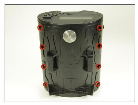
Using a Philips head screwdriver, remove the eight 6mm screws located at the bottom of the device.
