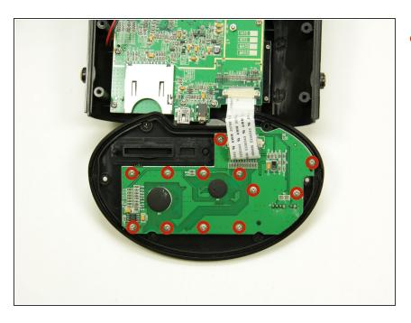
Using a Phillips head screwdriver, remove the twelve 3mm screws from the circuit board.
