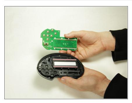
Gently remove the circuit board from the face of the camera.
