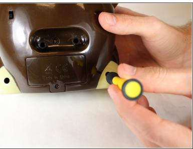
Remove all six 7.3 mm screws with a #00 Phillips head screwdriver.
