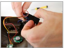
• Pull off the clock motor housing and un-clip the 4 clips on each side.
