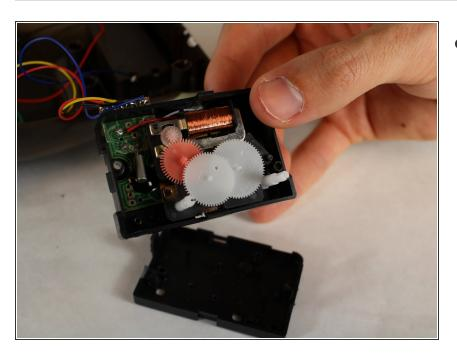
Repair any lose or misplaced gears or wiring.
