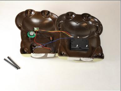
Once the clock is apart, carefully pull both halves until the clock is in two separate halves.
