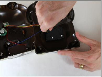
Unscrew the two 2 mm screws with a #00 Phillips Head screwdriver.
