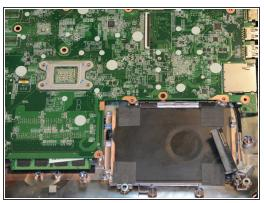
Locate and remove the silver hard drive cover in the bottom right corner.
