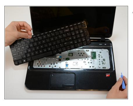
Once part of the keyboard has popped up, continue to lift the keyboard until it is removed.
