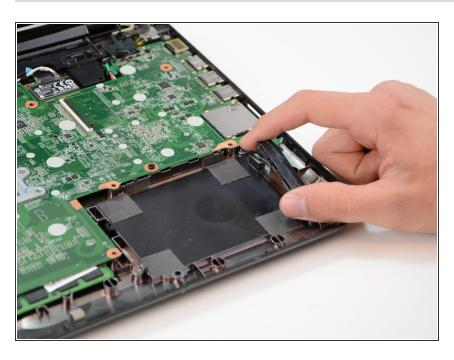
Detach and remove the hard drive from the black plug located to the right of the hard drive.
