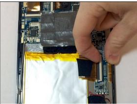
• There should be two cips that are also holding the motherboard in place, they should look similar to the one that held the camera in place. Unclip these the same way you did the camera.
